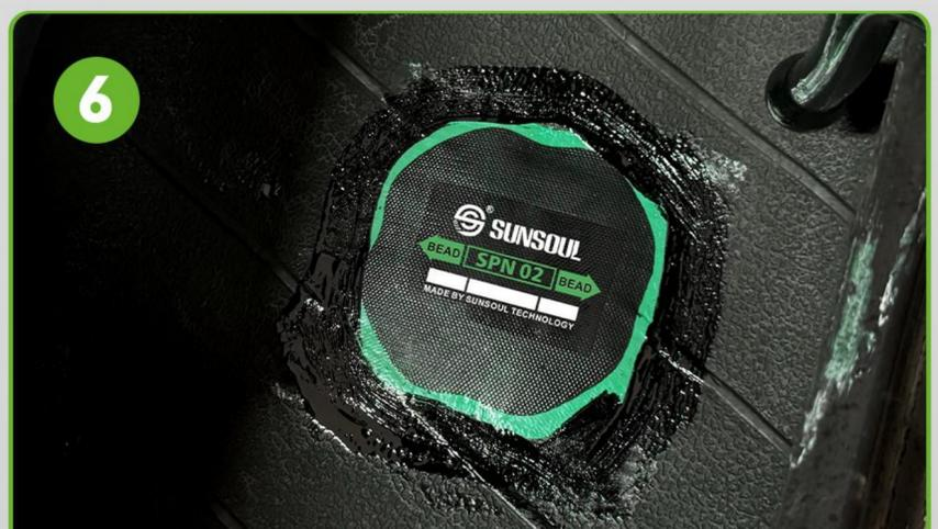
6 Apply innerliner repair sealant to the exposed buffed areas
