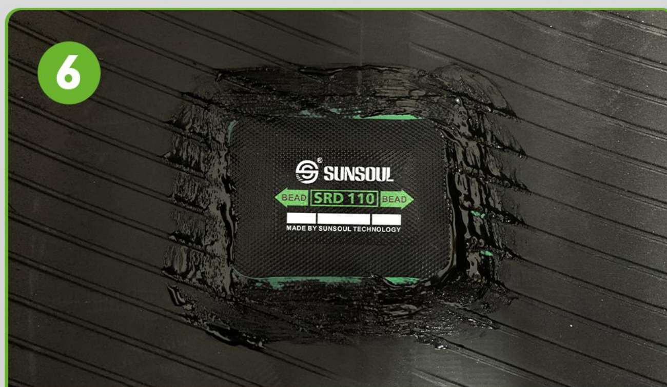
Apply innerliner repair sealant to the exposed buffed areas
