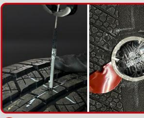
Grasp the wire with pliers on the outside of the tire and pull the stem through the tire until the cap forms a slightindentation.
