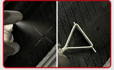
Pre-clean the inner liner 2 to 3 times with Rubber Cleaner and a scraper to remove contaminants.
