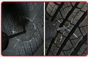
Damaged rubber and steel should be removed from the injury using a carbide cutter on a low speed air/electric drill. maximum 1,200 RPM. Drill the injury from the inside of the tire 3 to 5 times. Repeatthis process from the outside.
