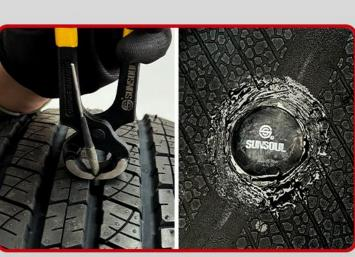
With the stem relaxed, cut off the excess stem 1/8"(3mm) above the tread surface.
