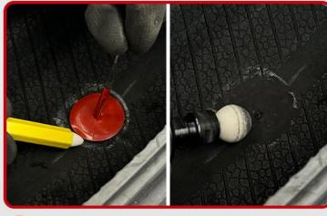
Outline the area to be buffed. Buff the outlined area with a low RPM buffer (Max 5,000 RPM) and appropriate inner liner wheel.
