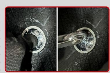
Press down the repair with your thumb from the center out. Stitch repair unit down from the center out. Remove blue poly from under cap and continue stitching toward the edge ofthe repair.
