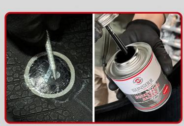
Remove the clear poly from the repair.
