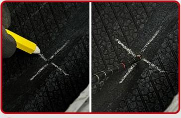
Locate and mark all damage on the inside and outside of the tire. insert a spiral cement tool or a probe into the injury from the inside of the tire to determine the size and angle of the injury.
