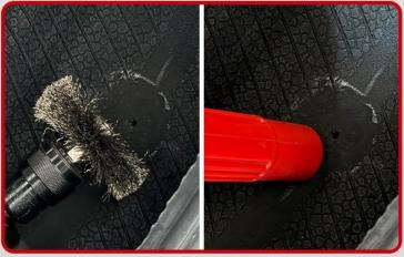
Use a soft wire brush followed by a vacuum to remove buffing dust and debris from the buffed area.
