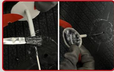
Apply a small amount of vulcanizing fluid to the black tapered portion of the stem. Insert the lead wire through the injury from the inside of the tire.
