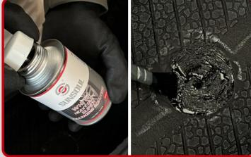
Using a spiral cement tool in a clockwise direction, apply Chemical Vulcanizing Fluid to the injury3- 5 times. Apply a thin, even coat to the buffed surface and allow to dry 3-5 minutes. Additional time may be required in cold or humid conditions.
