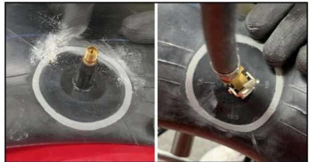
15 Apply White powder to the replacement valve. This will prevent the gray cushion gum from adhering to the tire. The tube is now ready to be returned to service.
