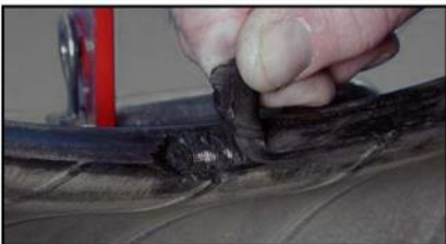
7. Deformed bead, exposed fabric or steel
