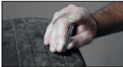
5. Excessive tread wear
