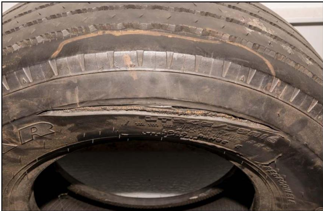
Zipper Rupture in a Light Truck Tire with steel body plies.
